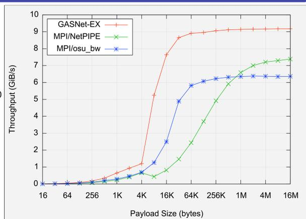
**Flood Bandwidth Graphs** report tests of achievable one-way bandwidth for point-to-point data transfer between two nodes.
