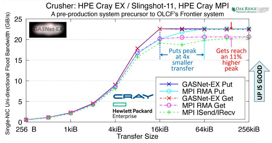
A comparison of uni-directional point-to-point host-memory flood bandwidth benchmarks, run March 2022 on OLCF's Crusher system. Shows the performance of RMA (Put and Get) operations using GASNet-EX and both RMA and message-passing (Isend/Irecv) using HPE Cray MPI. Results were obtained using then current GASNet tests and Intel MPI Benchmarks, respectively.
